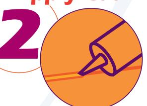
Slowly squeeze the trigger on the caulk gun, allowing the caulk to extrude from the cartridge or tube tip at the rate that is best for your work. Make sure the caulk comes in full contact with application surfaces. For best results, the caulk should not adhere to more than two permanent surfaces planes or sides.
